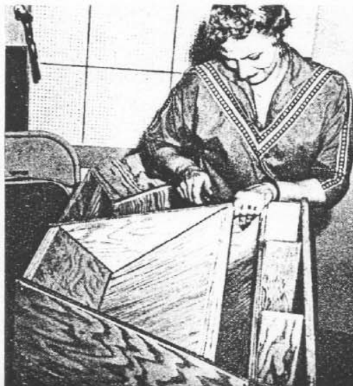
Fig. 25—Draw up screws till glue squirts out of joint top and bottom.
