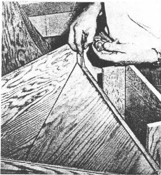
Fig. 21—Calking seams with Marine Glue.
