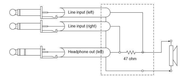
Figure 6. Cabling for impedance measurement using headphone output
