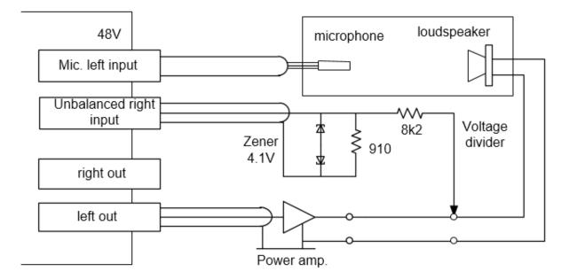
Figure 7. Cabling for two channel frequency response measurements
