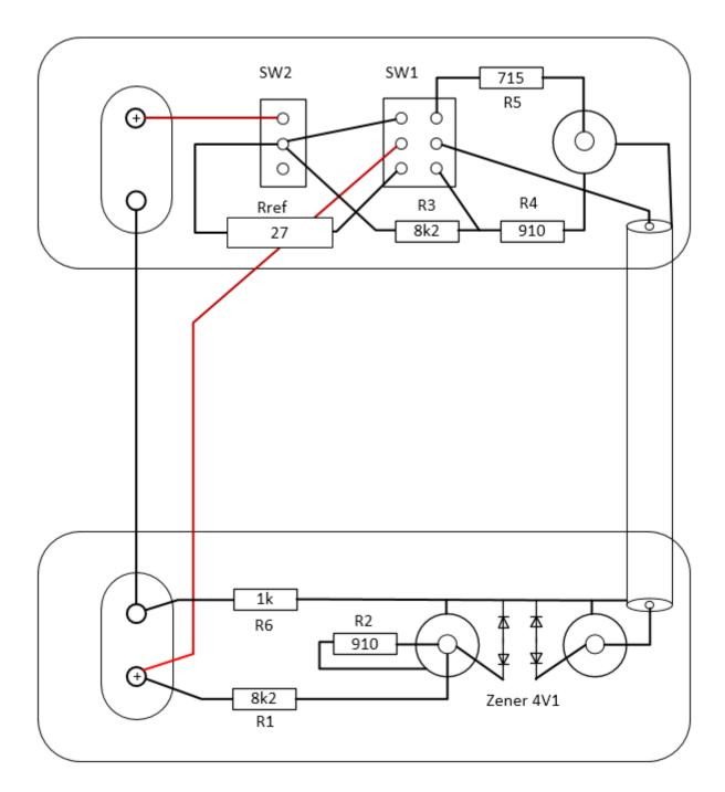
Figure 4. Connection plan for ARTA-Measuring box
