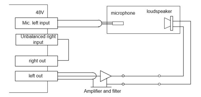
Figure 8. Cabling for crossover response measurements using semi two-channel setup (power amplifier passband gain must be entered in ARTA device setup)
