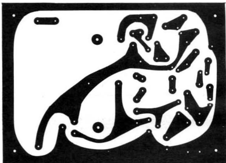
Fig. 5. Actual-size photo of amplifier printed circuit board can be copied or the board can be purchased etched and drilled (see note in Parts List).
