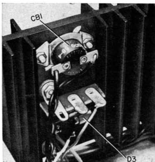
For proper operation, sensing element of thermal circuit breaker CB1 must contact Q7 's heat sink.
