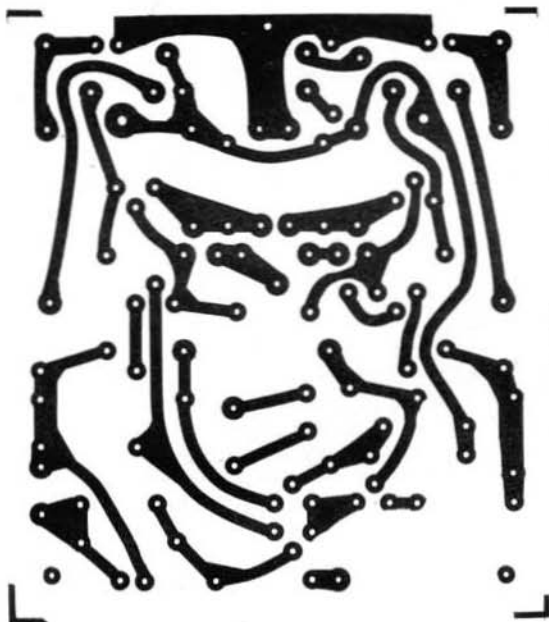
Fig. 5. Actual size etching and drilling guide at left is supplied for those who wish to make their own PC boards. Diagram above shows locations and orientations of components on PC board.
